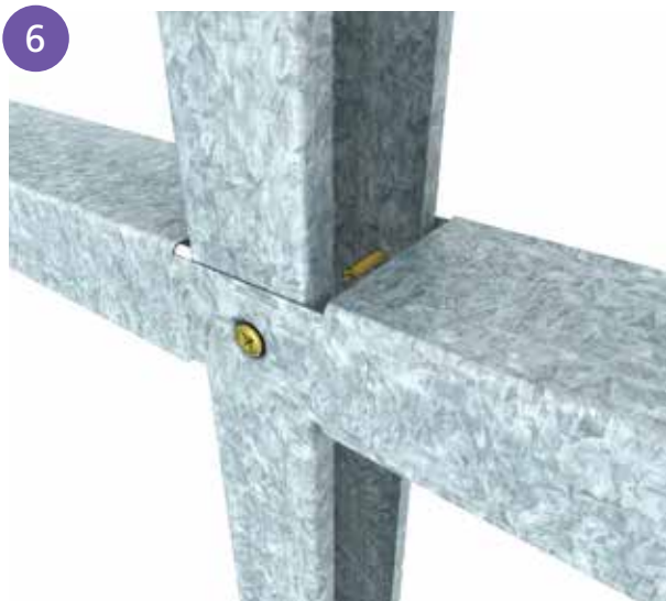
■ COMMON STUD NOGGING DETAIL
