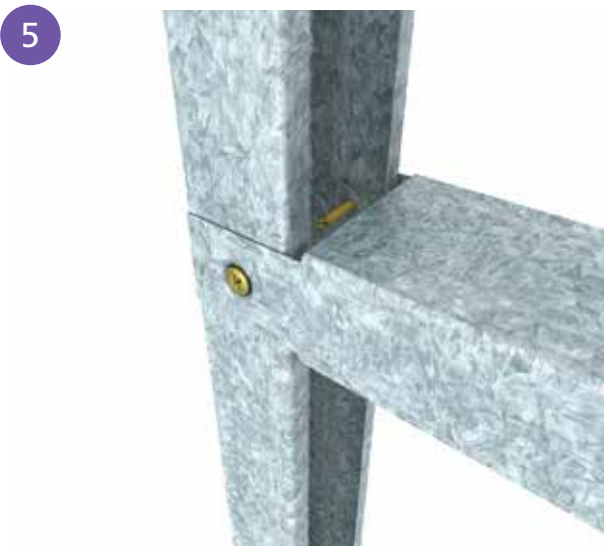
■ NOGGING TRACK END DETAIL
