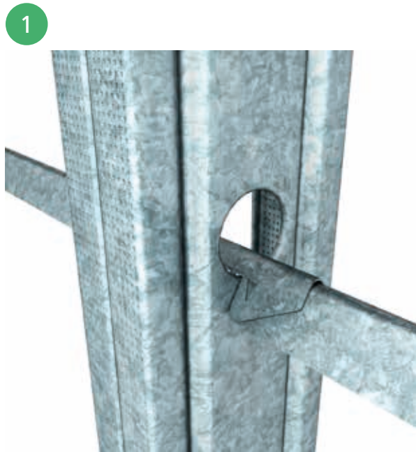
■ OVERLAPPING OF SNAP-LOCK NOGGING WHEN CONTINUOUS
