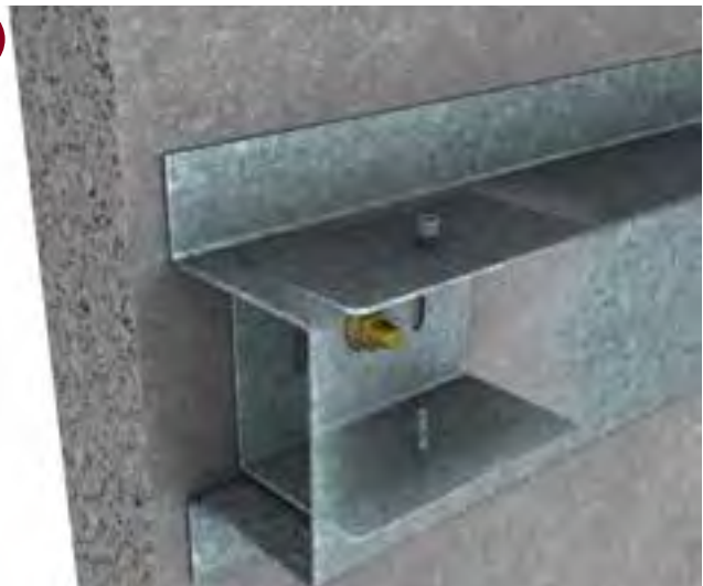
■ TOP HAT FIXED TO CONCRETE ANCHOR SIZE TO CONCRETE/MASONRY 8-10mm AS SPECIFIED. TOP HAT TO CLEAT WITH #12 TEK SCREWS AS SHOWN
