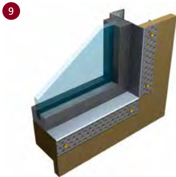
■ REVEAL BEAD INSTALLATION
